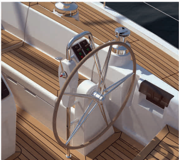
The 'standard' Xc 45 comes with stainless steel wheel crash bars. Optional enlarged crash bars with integrated engine throttle and/or thruster controls on the starboard wheel.
