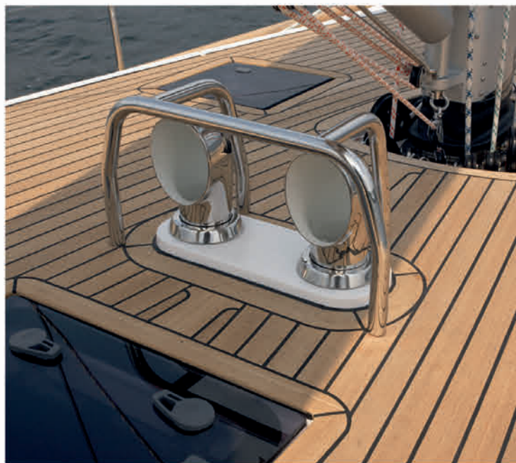
Stainless steel ventilation dorades are mounted on the coach roof, with stainless steel protection bar, provide excellent ventilation into the accommodation.
