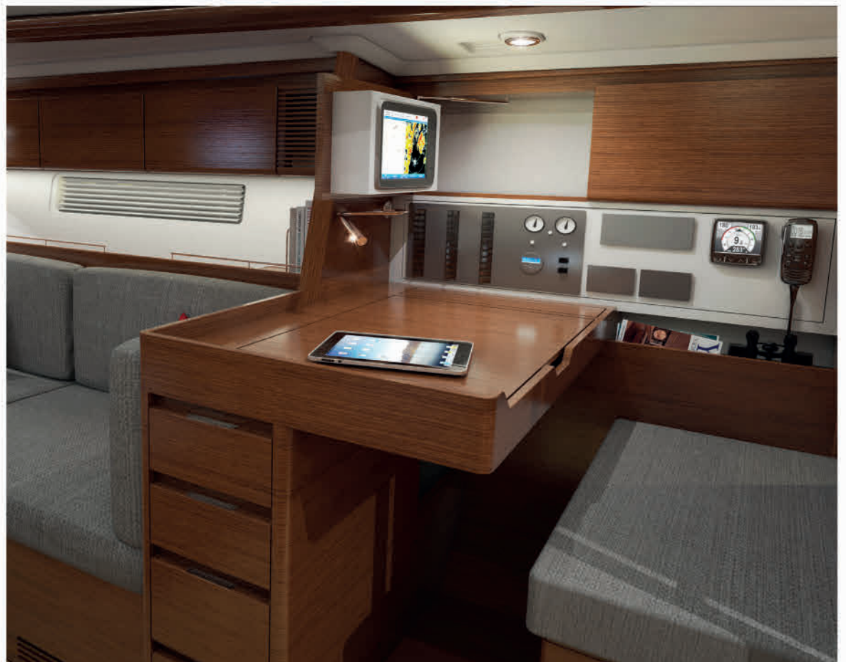
Right: The top cupboard "chart plotter" door in the open position. A gas spring holds the door securely in place when open.
