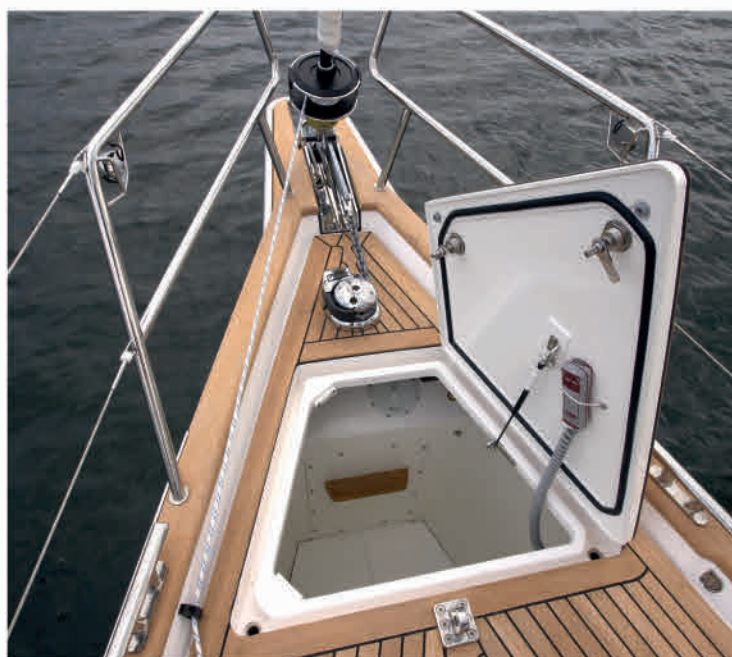
In the foredeck a deep sail locker, with integrated self-draining anchor chain compartment. The electrical anchor winch capstan can be fitted with an optional topwinch to operate moorings.
